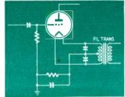
Fig. 15—How to bias a filamentary tube.
