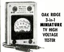
Accurately checks all high voltages in any direct-view or projection TV set. Has precision 10,000 ohm/volt movement, three scales: O-500V, O-15KV, O-30KV. Complete with special high voltage test lead. Size: 5½ x 4 x 2½". Dealer's Net \$14.95.
