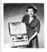
operating conditions, which takes relative tube life into account. Twelve sockets provide for testing four-, five-, six-, seven-, eight-, and nine-pin tubes; octal and lock-in miniatures; subminiature, acorn, and hearing-aid types; mobile and ruggedized tubes; and pilot lamps.
