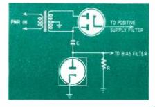
Fig. 5-Shunt diode reduces heat losses.
